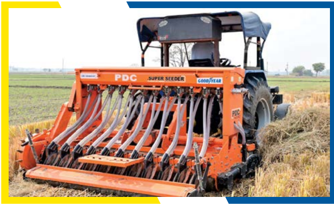
Farmer using Super Seeder for in-situ management of crop residue in Barnala
